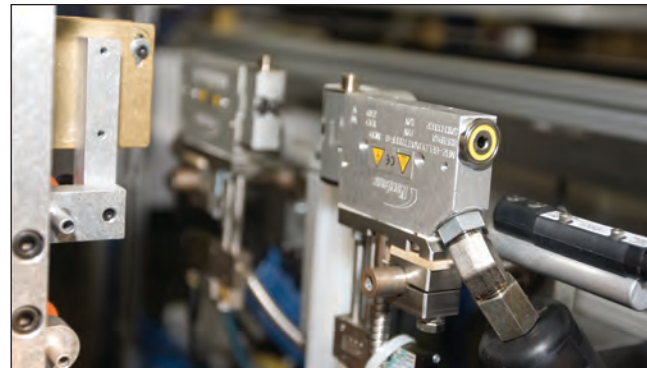
Optional Nordson hot melt paste attachment for additional adhesive in the joint area is available with our standard equipment: Cold Adhesive Pump and Regulator and Electronic Controlled Nozzle Spray for Precise Application. Multi-Language Touch Screen Control Panel
