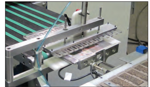
3. Book is aligned and ready for auto-feed transfer.
