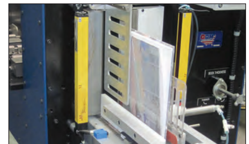
5. Electronic eyes align book, insuring a smooth transfer into Super Smasher™ for building-in process.
