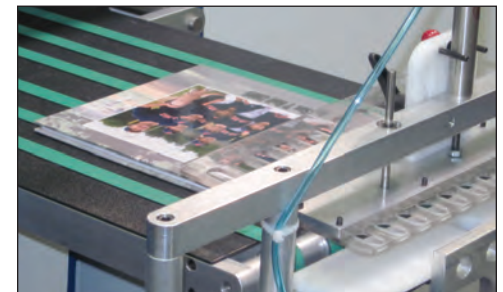
2. Hard cover book enters the gripping mechanism.
