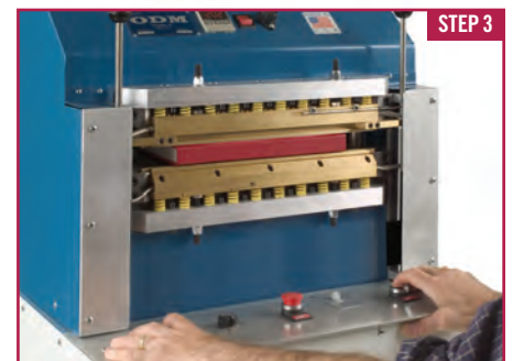
STEP 3 The book is clamped between two steel platens and the joint area is pressed with heated irons that help form the joint.
