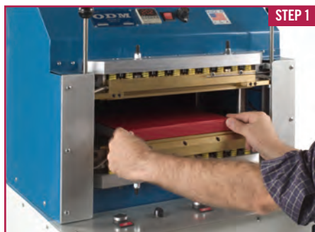
STEP 1 The operator places the cased-in book into the Smasher and steps on a foot pedal to find the joint area of the book.
