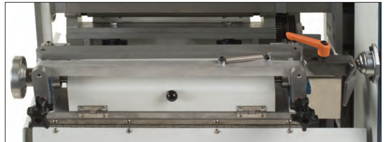
Extra paste attachment deposits additional adhesive in joint area.
