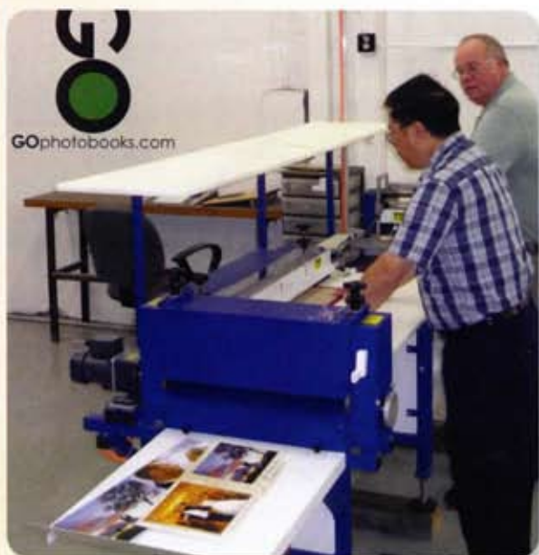
GPhotobooks.com's casemaking system from ODM will produce 120 to 200 hardcovers per hour when configured for two operators.
