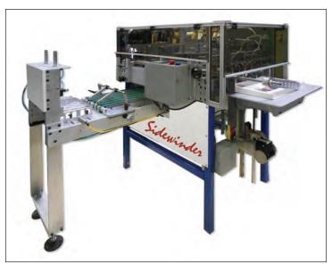
Sidewinder<sup>TM</sup> scores, folds, and presses Mohawk Panoramic papers allowing beautifully printed images to flow seamlessly across the fold, giving digital printers of all sizes the ability to produce high-value, high-impact books and bound products without a gutter.
