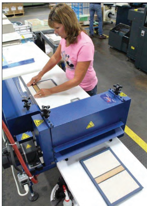
Casemaking System™ consists of four steps: 1. Spreader™ 3. Stomper™ 2. Slider™ 4. Squeezer™
