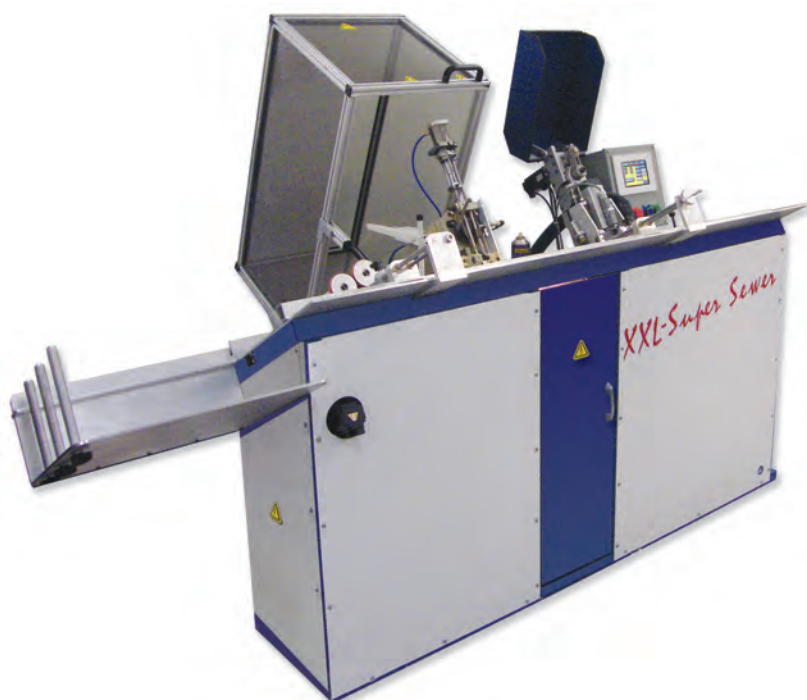
ODM Super Sewer™ XXL is ideal for side sewing tabloid size book blocks up to one-inch thick.
