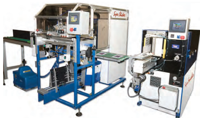
Super Sticker™ – an automated casing-in machine with Book-Trac™ for high volume bookbinding with transfer station.
