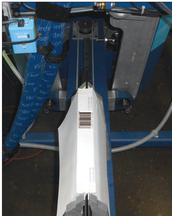
Operator just places the book block on the book carriage while the Super Sticker™ is in the home position. The ODM Book-Trac™ scanner reads the ID Barcode.
