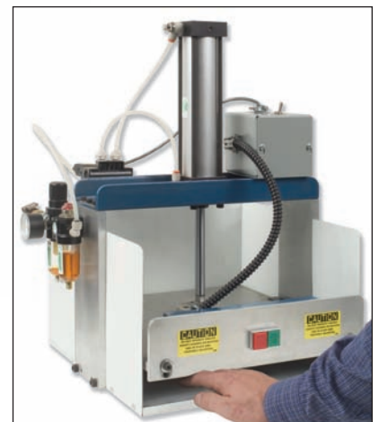
Micro switch sensor prevents hand injury.
