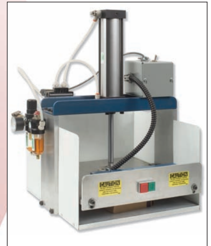
Air press squashing an accordion file folder.
