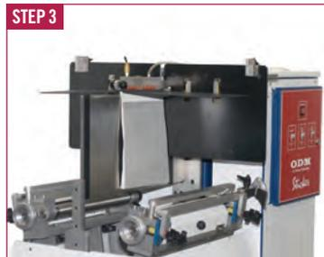
When the wing returns back to the home position, the cover guide bar is (manually) lowered to contact the spine of the book block.
