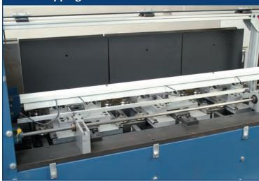
After the books are pressed in the smashing station, the books travel through three nipping stations (a safety guard box lifts open for easy access to joint irons located in the rear of the machine) that apply up to 1,500 pounds of hydraulic pressure to the joint area of each book. The three nippers provide dwell time in the joint area enabling the machine to run at speeds up to 18 books per minute.
