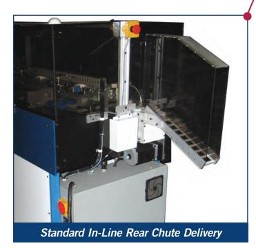
The standard in-line rear chute delivery of finished books can be tied into most conveyor systems for continuous work flow.
