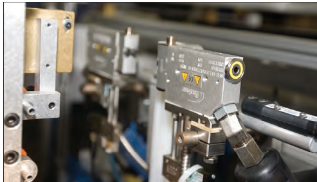
Optional Nordson hot melt paste attachment for additional adhesive in the joint area is available with our standard equipment: Cold Adhesive Pump and Regulator and Electronic Controlled Nozzle Spray for Precise Application.
