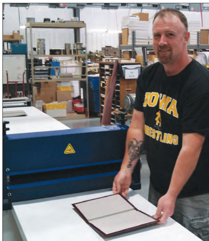
During the final step of casemaking, the finished cover is fed through the rotary squeeze press where the cover is pressed to insure the cover material and boards are laminated.
