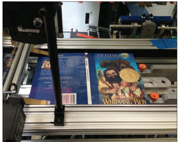
Book covers are stacked on the left conveyor belt and the ODM Book-Trac™ scanner prior to casing-in process reads ID Barcode.
