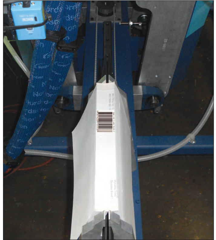
Operator just places the book block on the book carriage while the Super Sticker™ is in the home position. The ODM Book-Trac™ scanner reads the ID Barcode.
