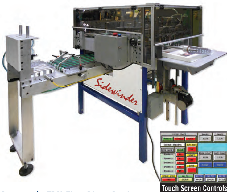
Convertible Solutions' TRU-Flat® binding technology produces 27" x 14" (open) lay-flat photo books up to 1" thick.
