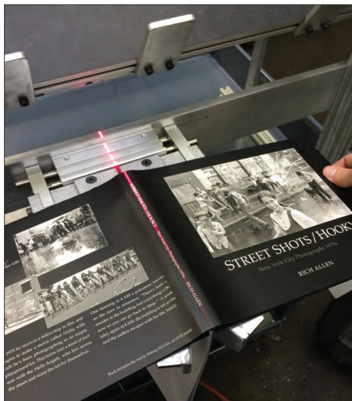
Laser centering line is used to line up the printed book jacket on the spine of the book.
