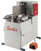
is placed on a "wing," the operator hits a foot switch and the wing drops below the glue rollers; the rollers apply glue to the endpapers; and the hardcover is placed in position.
