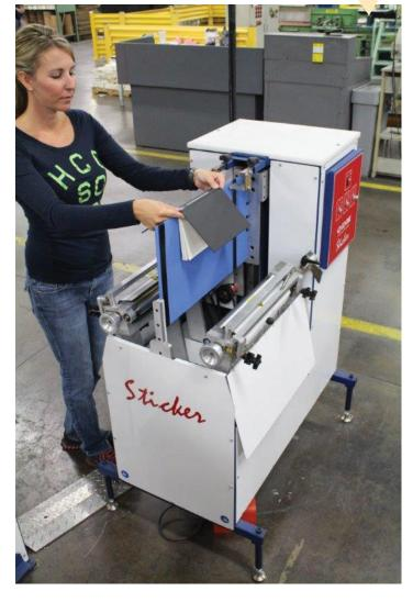
Different binding equipment is better suited to different output levels. ODM's digital hardcover binding equipment shines in the short (1-750) run and has low makeready time. Especially when handling short and ultra short runs, make-ready time can be the difference between a cost effective solution and a cost prohibitive one, says Jacobson. "If you have to do make ready for two or three sheets, you have that whole cost allocated over a small number of units, your price obviously balloons."
