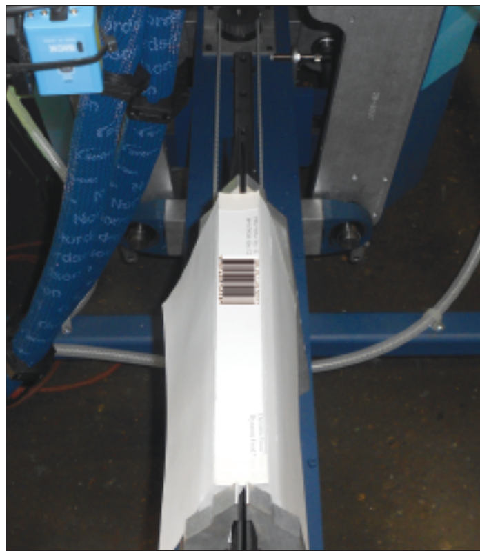
Operator just places the book block on the book carriage while the Super Sticker™ is in the home position. The ODM Book-Trac™ scanner reads the ID Barcode.
