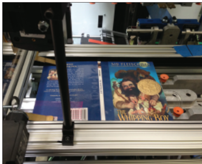
Book covers are stacked on the left conveyor belt and the ODM Book-Trac™ scanner prior to casing-in process reads ID Barcode.
