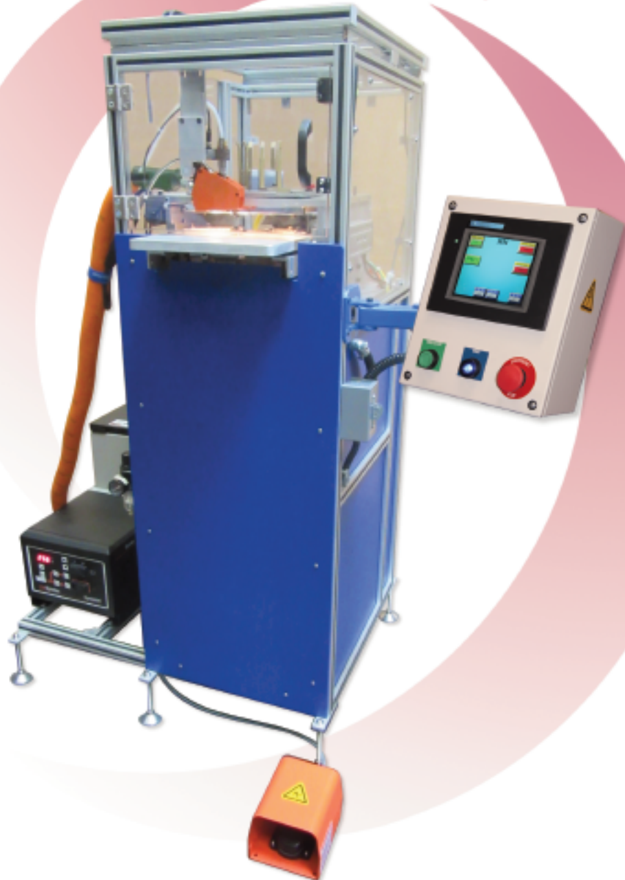
Menu panel is hand inserted into precision guides prior to depressing foot pedal cycle for panel corner application.
