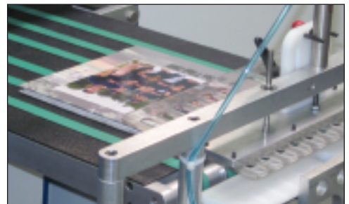
2. Cased-in book enters the gripping mechanism.
