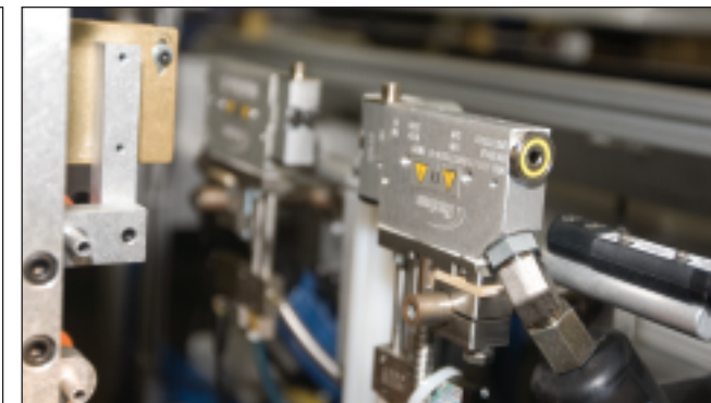
Optional Nordson hot melt paste attachment for additional adhesive in the joint area is available with our standard equipment: Cold Adhesive Pump and Auto Adjust Nozzle Spray for Precise Application. Multi-Language Touch Screen Control Panel
