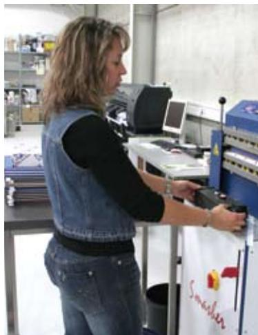
**Above right:** During casemaking, the hard cover is produced in four simple steps: Spreader, Slider, Stomper and Squeezer. First, the cover material goes through the top side gluer (Spreader), then the operator spots and aligns hard cover boards in position with the sliding table case gauge, shown above (Slider). All four sides of the hard cover are turned-in, see insert (Stomper). Finished hard covers go through the rotary press (Squeezer).
