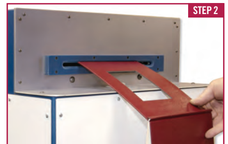
Operator Depresses The Foot Pedal That Die Cuts A Window
