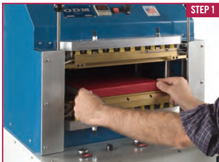
The operator places the cased-in book into the Smasher and steps on a foot pedal to find the joint area of the book.
