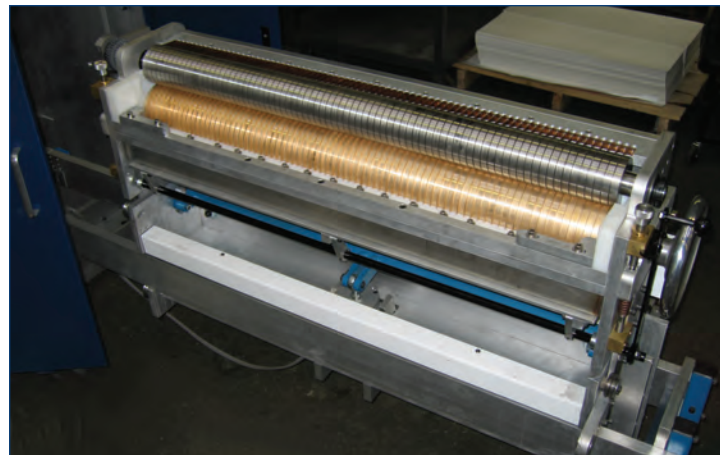
Heavy-duty gluer roller slides out for easy access and fast clean-up.
