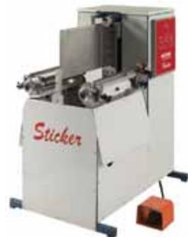
The Smasher™ is a building-in machine. The cased-in books are taken from the Sticker™ and placed in the Smasher™. The operator locates the joint area, and then activates the hydraulic system that clamps the book with 20,000 pounds of pressure. Heated joint irons help form the joint by melting the adhesive in the joint area. The Smasher™ has an adjustable dwell timer that controls how long the book remains under pressure.
