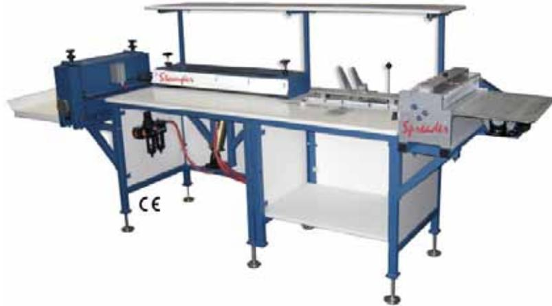
Step 2: Once adhesive is applied to the cover material, the Slider aligns the hardcover boards in position. The Slider’s arms open as wide as four inches, and the unit also comes with an adjustable side guide and arm spacer kit for different joint gaps.
