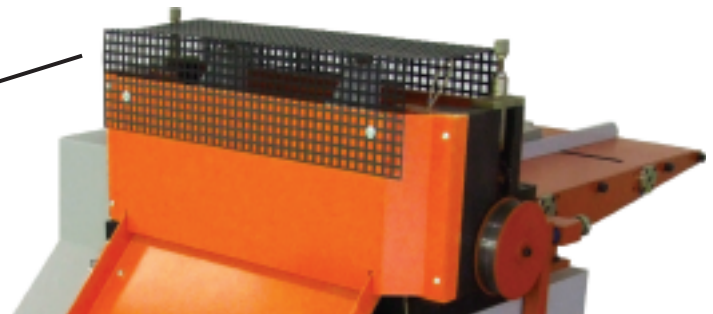
Cardboard automatically cut into strips for casemaking.
