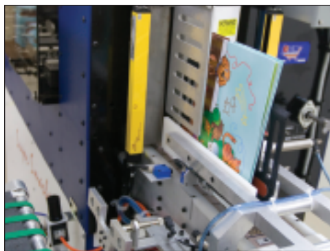
Hard cover book is lifted 90° into an upright position and loaded into Super Smasher™ via conveyor belt.
