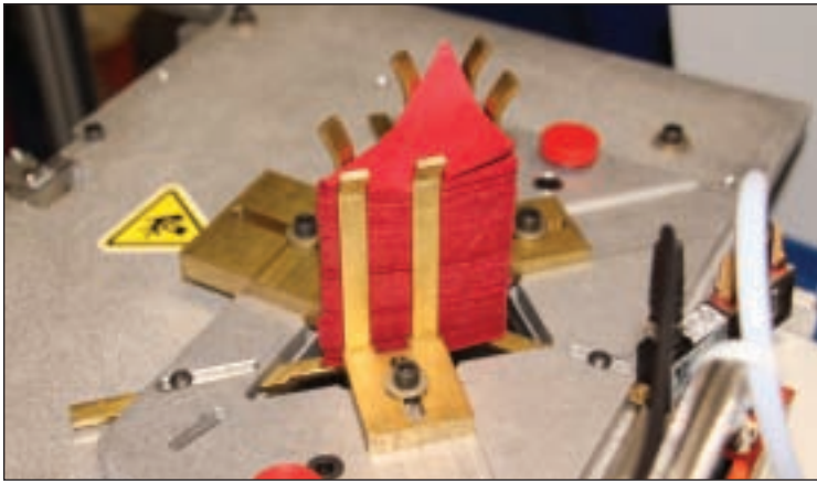
Top loading hopper stacks and pre-aligns corners. Holds up to 200 die cut corners.
