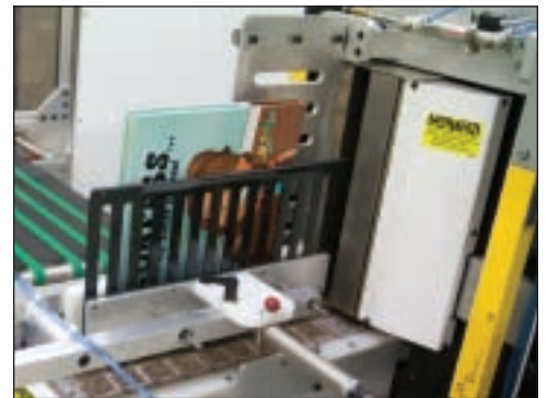
Electronic eyes align book, insuring a smooth transfer into Super Smasher™ for building-in process.
