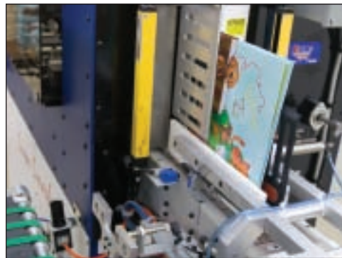
Hard cover book is lifted 90° into an upright position and loaded into Super Smasher™ via conveyor belt.
