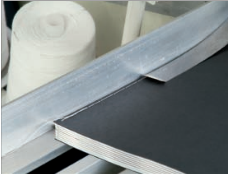
Back Tack Technology™ ensures a strong, side-sewn block with a reverse back stitch on the head and foot of the book block.
