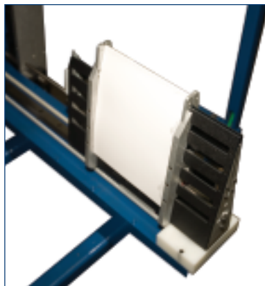
Operator places sewn book block on the wing, while in the 'home' position.
