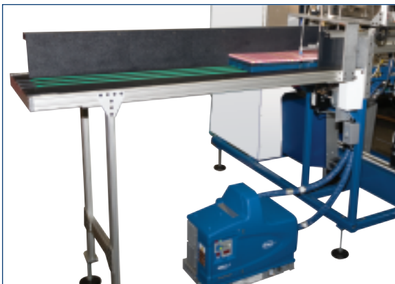
Operator places book covers on the left conveyor belt. Optional Nordson hot melt attachment shown below conveyor belt.
